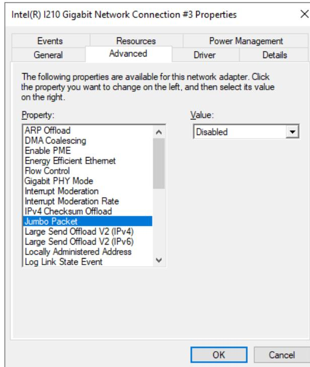
**Step 3.** Select the "Jumbo Packet", settings, and select the expected jumbo frame size and then go "OK" Finish.
