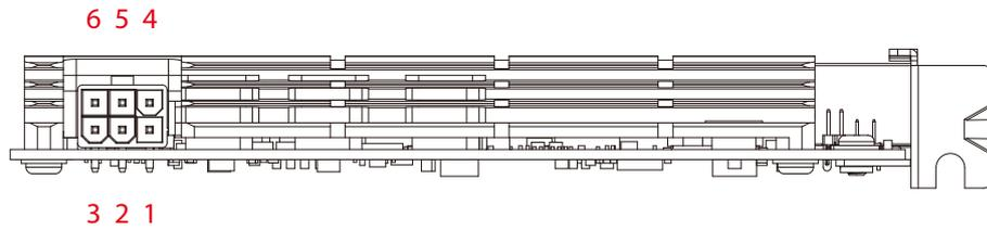
PE-2001H requires an external 6-pin power supply by default to support PoE Power supply.
