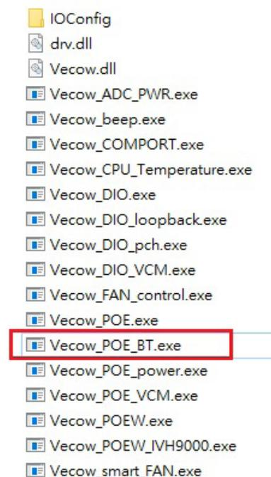
PE-2001H default is Auto power detect mode, you can use the following software control to switch to manual mode.
