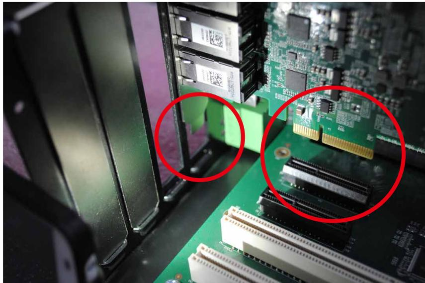
**Step 2.** Make sure edge-finger and PCI Express I/O bracket are inserted smoothly.
