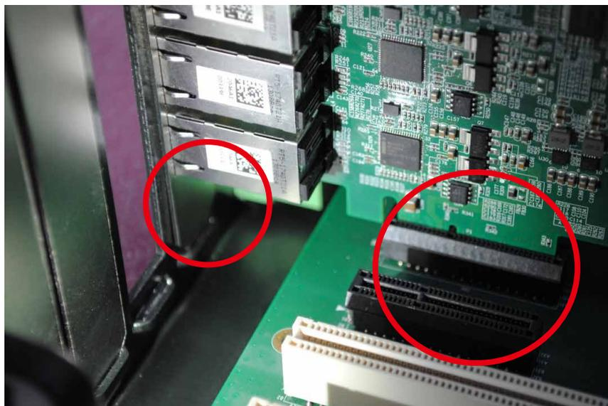
**Step 3.** Make sure PCI Express I/O bracket aligns screw hole.
