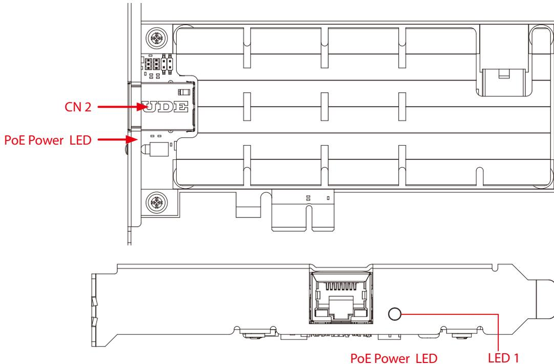
PE-2001H is equipped with one IEEE 802.3bt PoE++ ports for transmitting power as much as 90W / 54V per port and 10/100/1000Mbps data signals over standard Ethernet CAT-5/CAT-6 cable.
